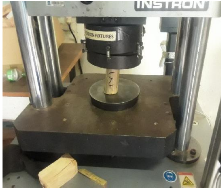
Figure 2: Specimen Undergoing Compressive Strength Test.
