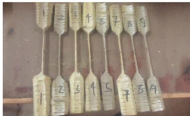
Figure 3: Specimens for Tensile Strength Test.
