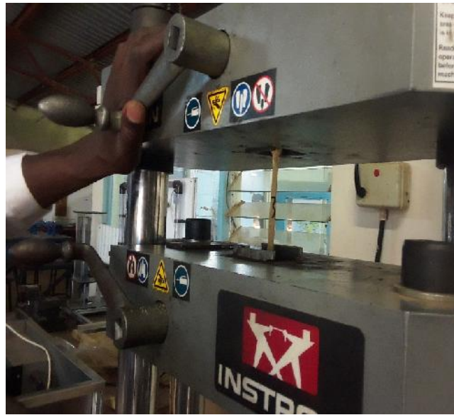
Figure 4: Specimen Undergoing Tensile Strength Test.
