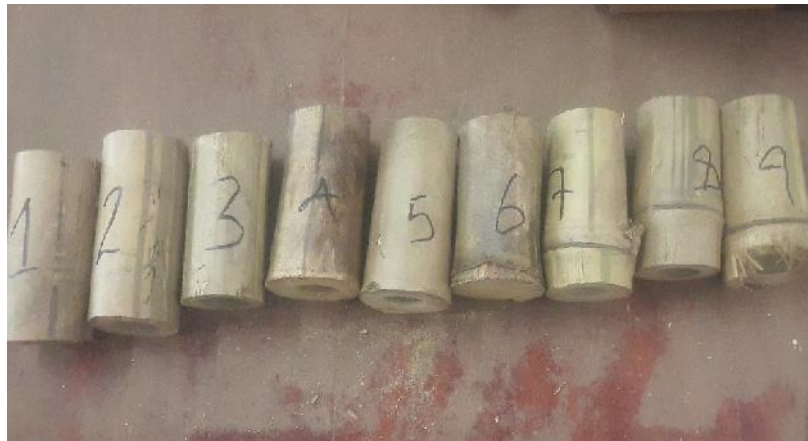
Figure 1: Specimens for Compressive Test.
